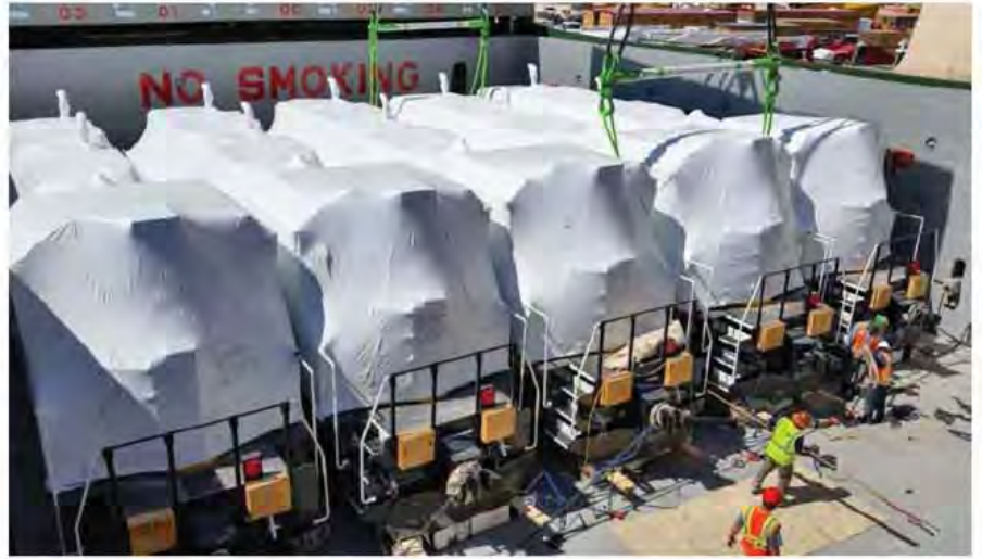
Railserve individually shrink-wrapped its locomotives to protect their exteriors from undue damage during transportation.
